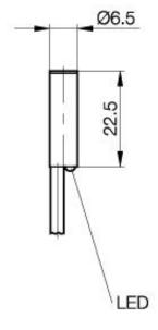
Inductive Sensors BES 516-371-SA 10-PU-03 D6.5 x 22.5 normally-open Sn=1,5mm shielded
